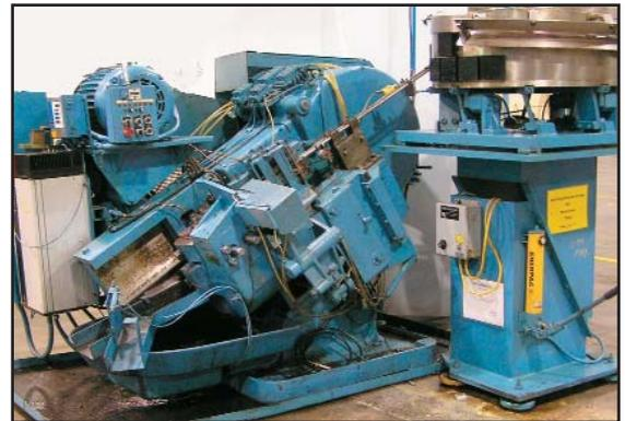
**WATERBURY FARREL #30** incline thread roller
