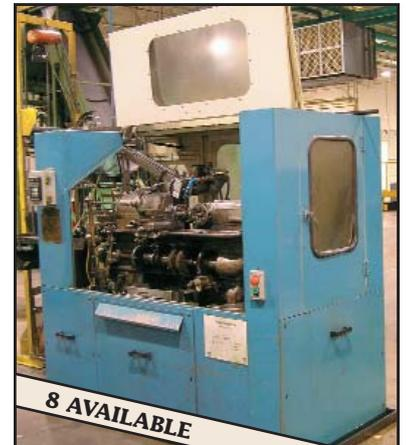
**BROWN & SHARPE 2G** single spindle automatic screw machine
