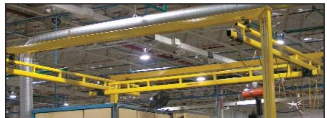
**LOADRAIL** 1 ton free standing crane system
