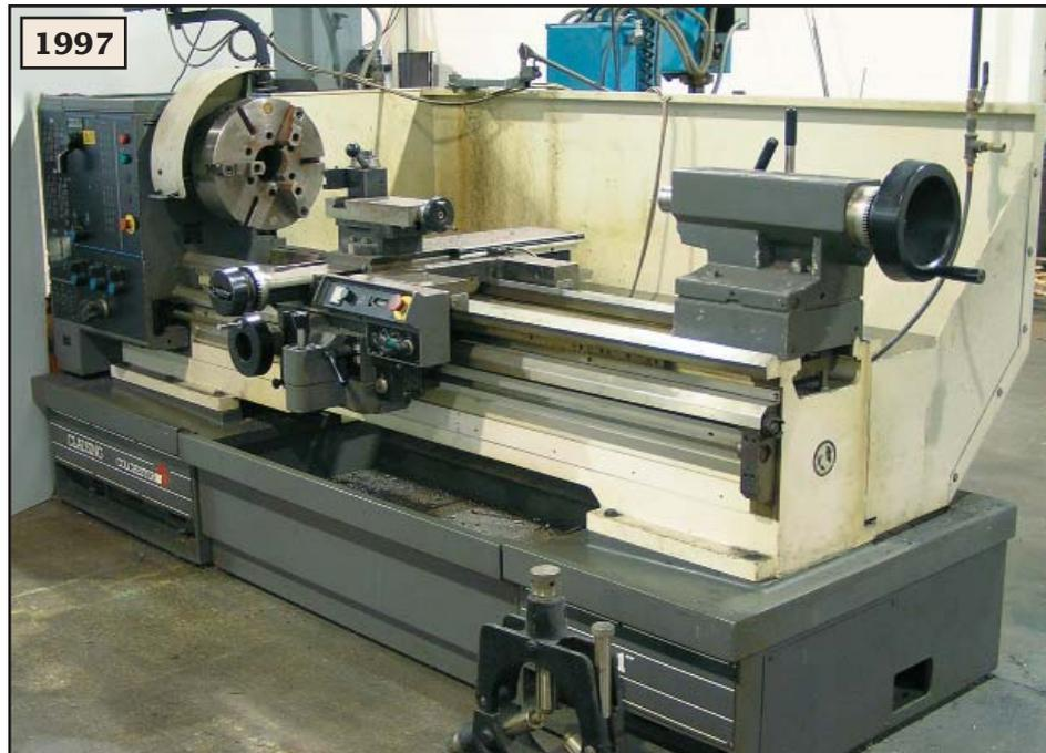
**CLAUSING/COLCHESTER MASTIF** VS engine lathe
