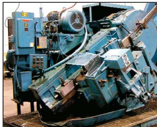
**WATERBURY FARREL #50** incline thread roller
